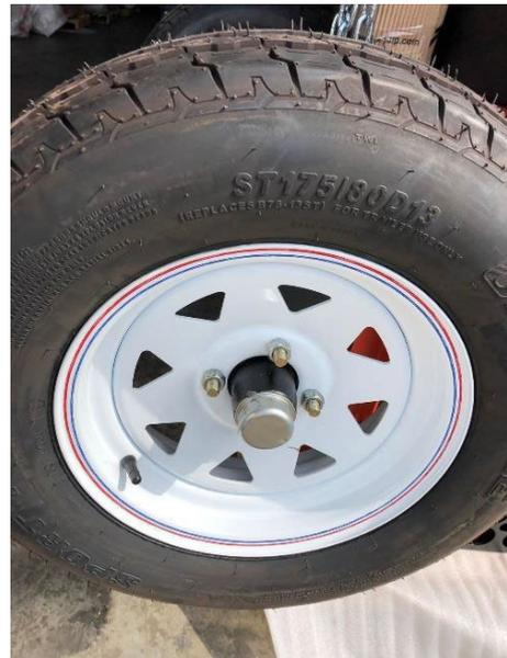
5. Once wheels are fastened proceed to remove hardware that holds machine to pallet using a 9/16" wrench and/or deep socket.
