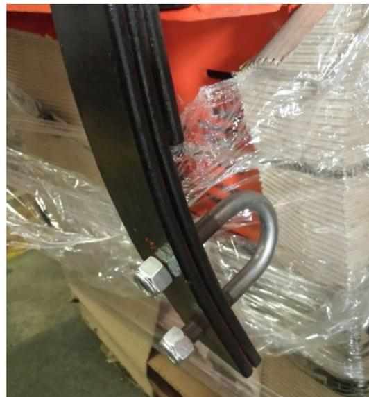
3. Remove the hex nuts on the U-Loops and place the axle through the loops then reinstall and tighten the hardware. The axle guides can be facing front or rear, make sure the axle guide is inside the U-Bolts before tightening.
