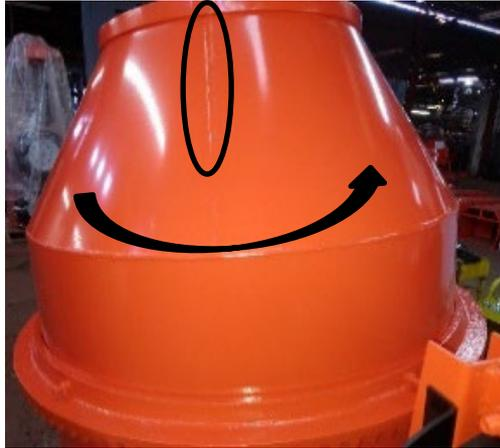
3) Locate the Weld line of drum and with the engine running at high speed, and the drum turning, count the number of turns per minute.
