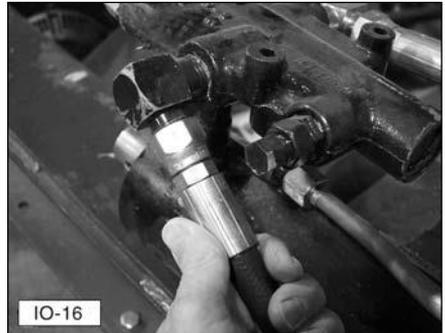
15. Coat the threads of the fitting with a hydraulic pipe sealant and attach the high-pressure hose from the bottom valve fitting to the pump, as shown. Securely tighten the hose fitting.
