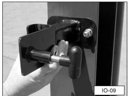
8. Block the wheels to prevent the base unit from moving. Carefully lower the rail assembly to a horizontal position. Securely tighten the nuts holding the base unit to the rail assembly (Step 5) and the nuts holding the rail rest assembly (Step 6).
