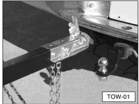
2. Release the latch assembly on the hitch coupler and lock the hitch coupler onto the tow ball. Attach the towing safety chains to the tow vehicle.
