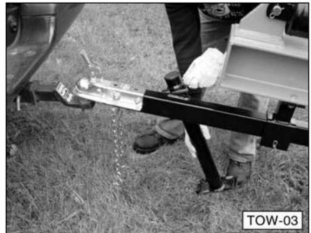
4. Place a customer supplied lock or lock pin into the latch assembly of the hitch coupler.
