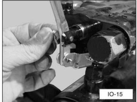
14. Attach the high-pressure hose from the filter assembly to the fitting on the side of the valve. Securely tighten the hose fitting.
