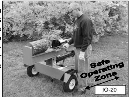
1. Set your log splitter on flat, dry ground. Make sure you read all the recommendations from the “Safety” section before using the log splitter.
