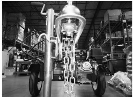
10. Place the hitch over the attachment tube, aligning the bolt holes, and insert the rear 1/2-13 x 3-1/2 inch bolt (A). Install and tighten the locknut.
