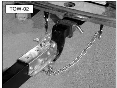
3. Raise the front leg to the towing position by pulling the spring pin. If not already secure, make sure the hitch coupler is properly and securely attached to the tow ball.
