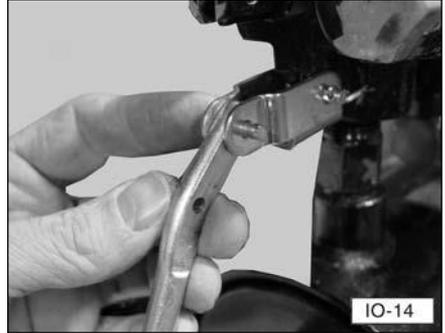
13. Attach the valve handle to the valve spool using a 1/4 x 1 inch long clevis pin. Secure the clevis pin with a cotter pin (bend the ends of the cotter pin to make it secure). Attach the knob to the valve handle, if necessary.
